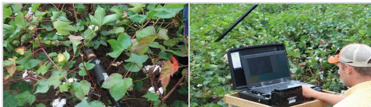
Figure 3. The MiniRhizotron camera (left) and image capture software (right).
