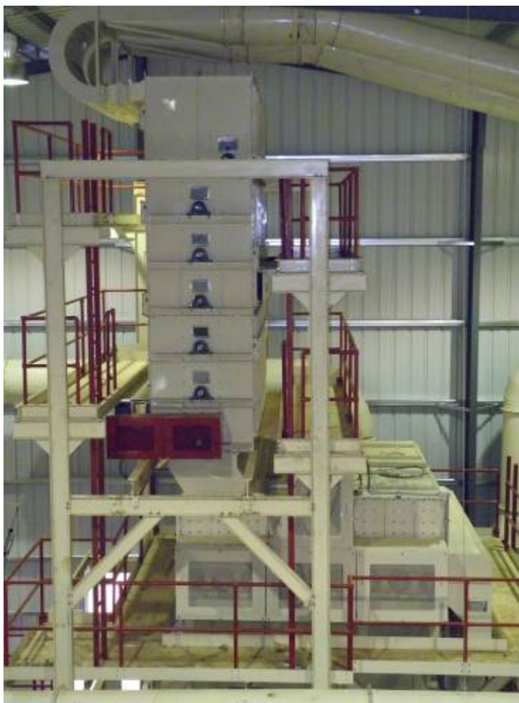
Figure 6. Vertical Cylinder Dryer Dooly Gin Lilly, GA
