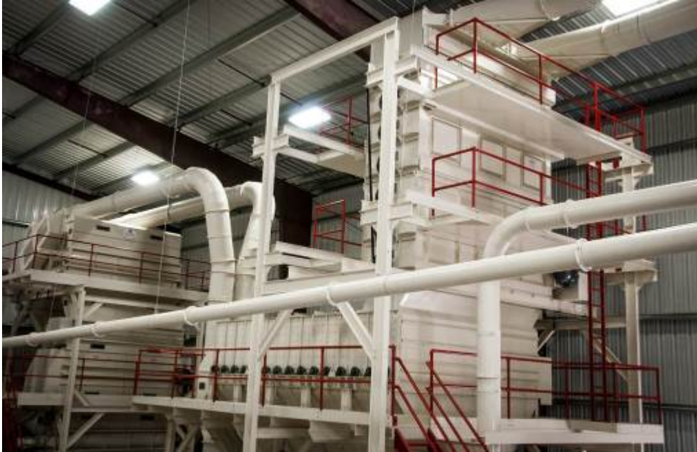
Figure 7. Vertical Cylinder Dryer over a 15 Cylinder Gravity Cleaner at Bernie Farmers Gin in Malden, MO.
