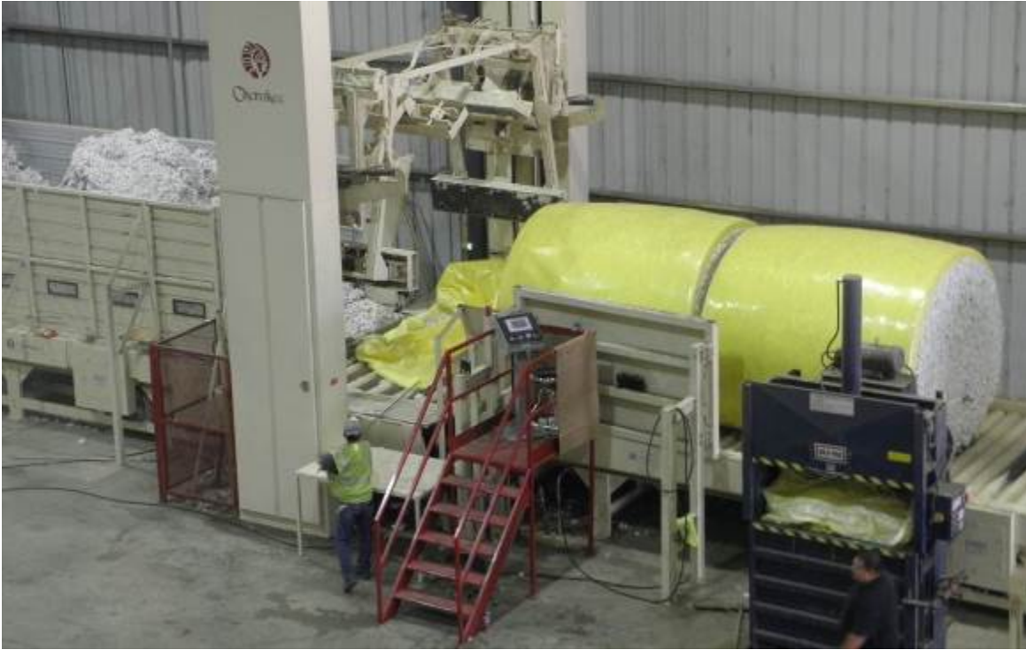
Figure 4. Operator Removing Wrap on a Round-Up II.
