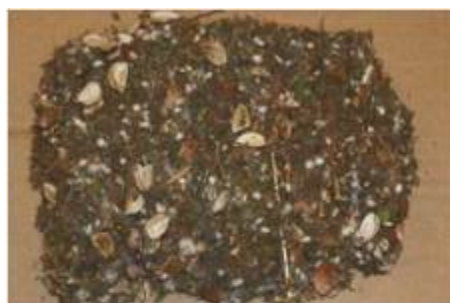
South Plant Stick Machine Trash
