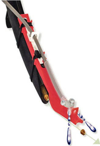
Figure 2. Image depicting the operation of the Schaffert Manufacturing “Rebounder” seed-firming system with application of material utilizing the “Y” splitter. This system delivers liquid material to the sides of the seed trench and was utilized in these trials to apply flutriafol in the modified in-furrow treatment in 2013 at both Coolidge and Solomon.
