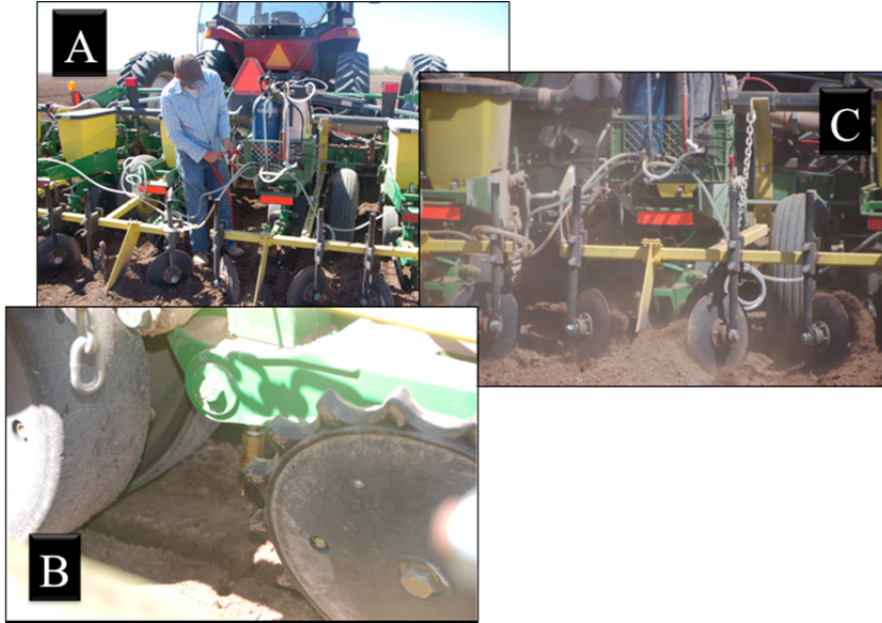
Figure 1. Images illustrating the application of flutriafol for trials in both 2012 and 2013 for the T-band and in-furrow treatments (IFT – not shown). A CO 2 pressurized spray system was attached to the planter (A) with nozzles attached in such a way as to apply a T-band over the seed trench (B). The system was calibrated at normal tractor operating speed to apply 4 gallons of material per acre with flutriafol rates of 16 and 32 oz/acre in 2012 and 32 oz/acre in 2013 (C).
