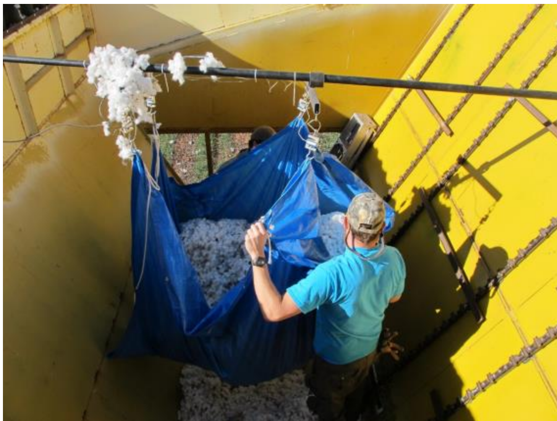
Figure 2. The sample collection system, located inside of the boll buggy.
