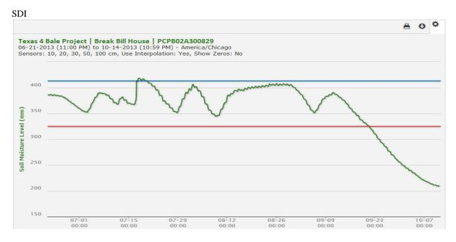
FC graphs indicate that SDI irrigations maintained soil moisture in the desirable range of readily available soil moisture without causing stress from low or excess moisture. In addition, during irrigation events water did not move through the lower part of the soil profile below 40 inches.
