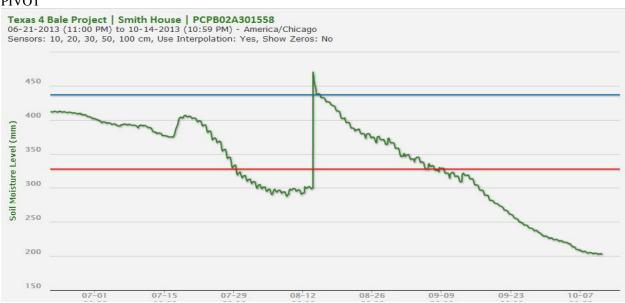
The FC graphs indicate that producer managed Pivot irrigations allowed the soil moisture level to drop below the refill line reducing the availability of soil moisture needed by the plant at a critical midseason timing. The corrective irrigation event resulted in excess moisture moving through the soil profile at 40 inches and slowed the uptake of moisture for approximately 24-48 hours due to excess water needed to refill the profile.
