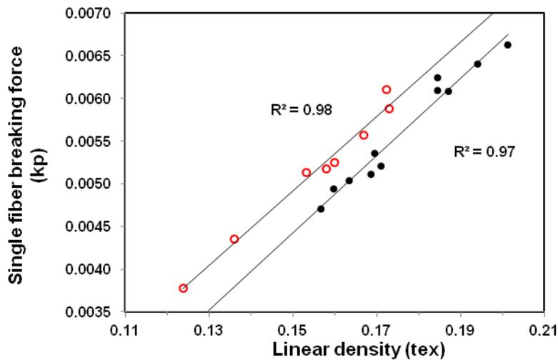
Figure 8. Relationship between single fiber breaking force and linear density among fine (○) and coarse (●) fibers ( $R^2 = 0.90$  for all samples).
