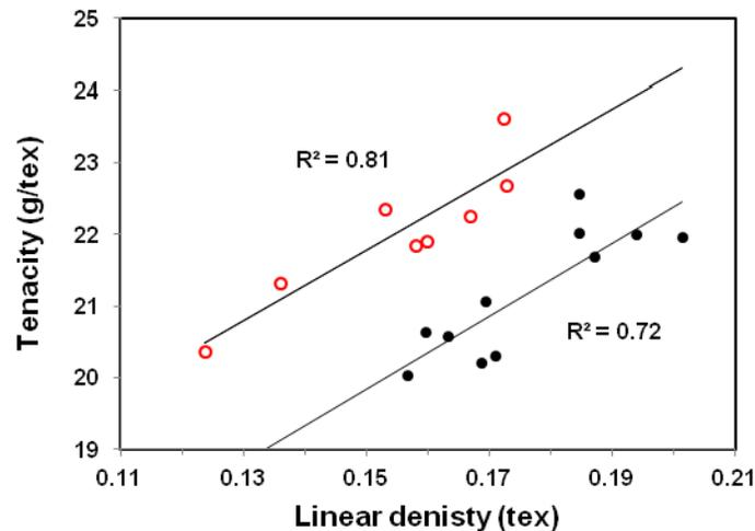
Figure 6. Representation of Figure 5 with two subsets of fine (○) and coarse (●) fibers.
