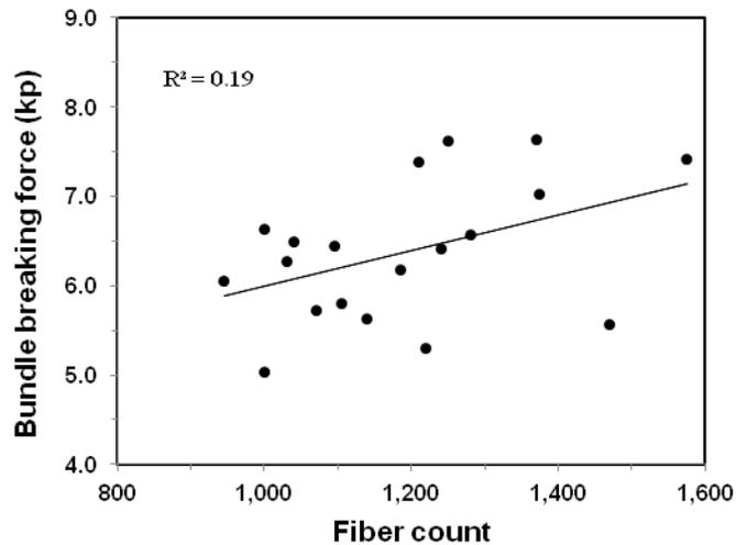
Figure 4. Relationship between fiber bundle breaking force and fiber count.
