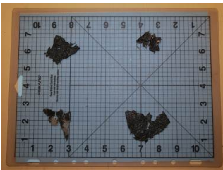
Figure 2. Dark plastic material found in a bale of U.S. cotton by a mill. Courtesy of Lance Murchison, National Cotton Council.
