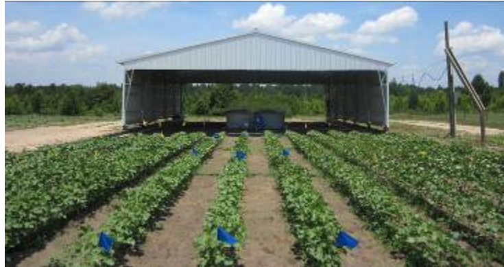
Figure 1. Automated rainout shelter.
