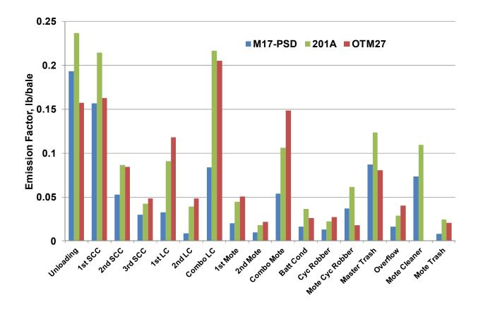
Figure 1. Average measured  $PM_{10}$  emission factors from EPA Method 17 multiplied by the percent less than 10 microns from the particle size analysis, Method 201A with only the PM10 sizing cyclone, and Method 201A with both the  $PM_{10}$  and  $PM_{2.5}$  sizing cyclones.
