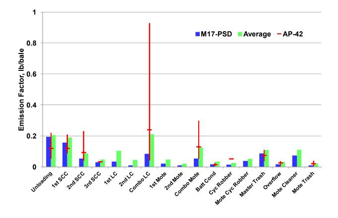
Figure 2. Average measured  $PM_{10}$  emission factors compared to EPA AP-42 emission factor averages (horizontal, red bars) and ranges (vertical, red error bars).
