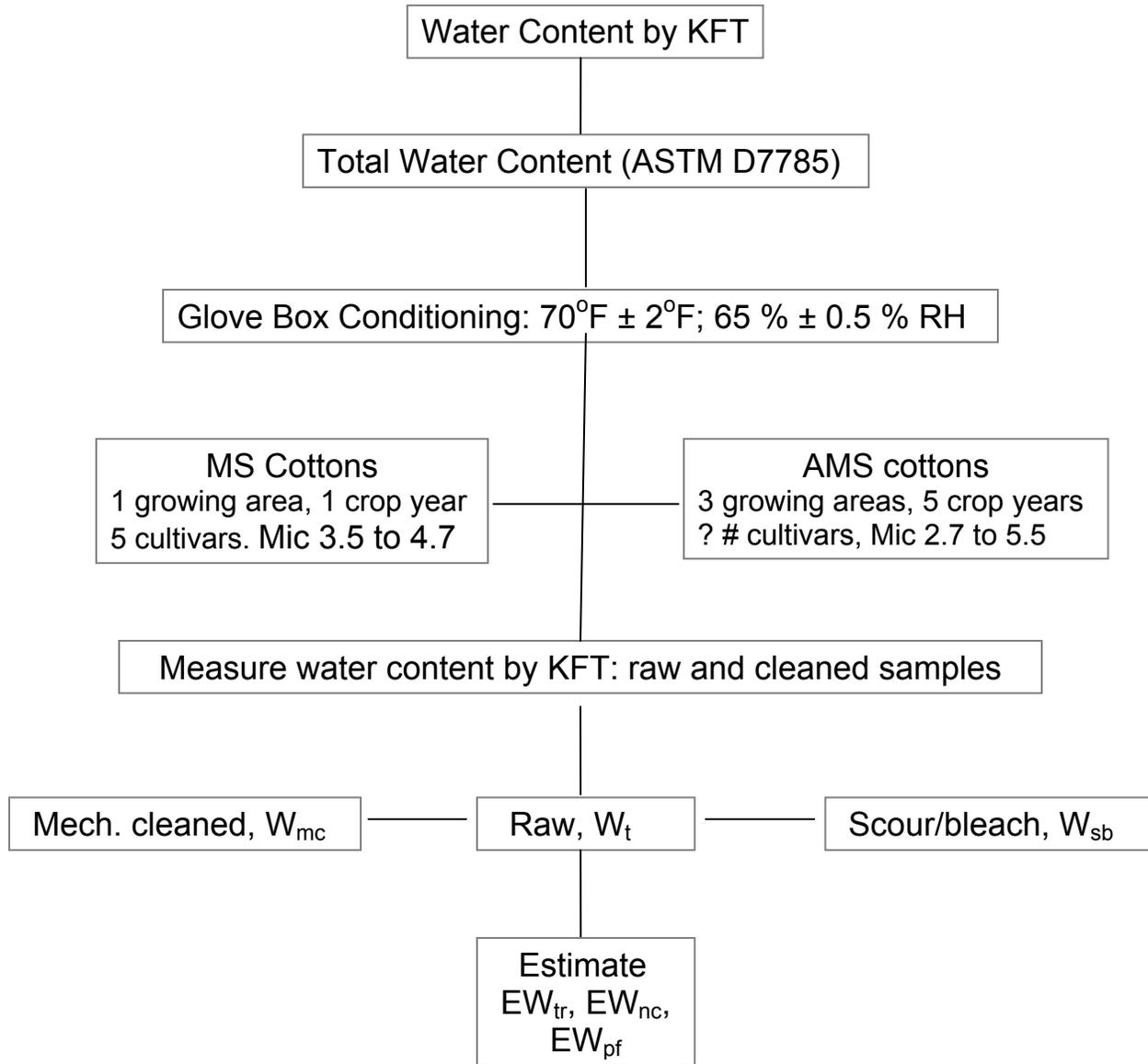
Figure 1. Flowchart of water content measurements.
