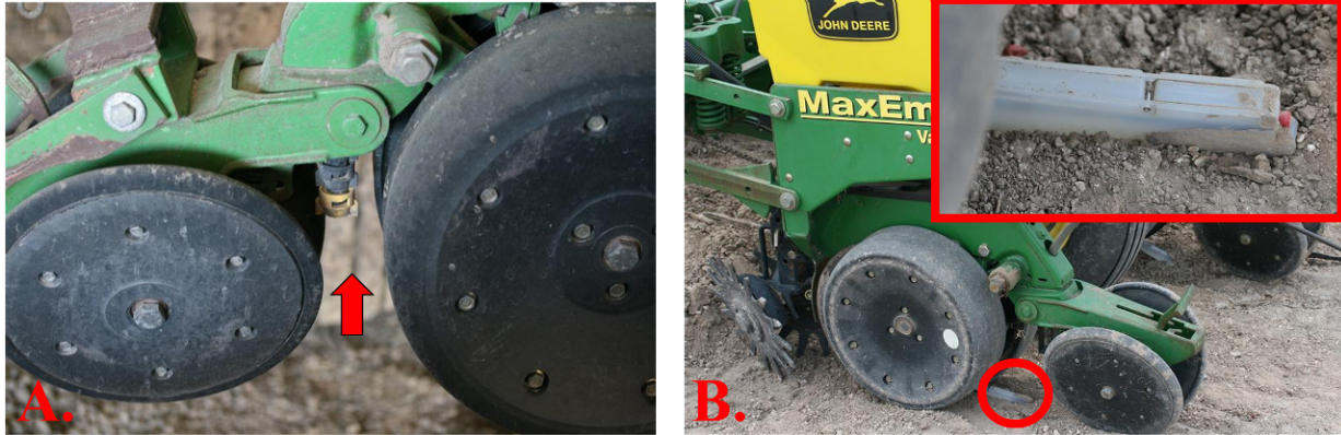
Figure 1. Application at planting. A. Placement of nozzle for T-band application (arrow). B. Nutramark seed bed firmer used for in-furrow application (circled and detail).
