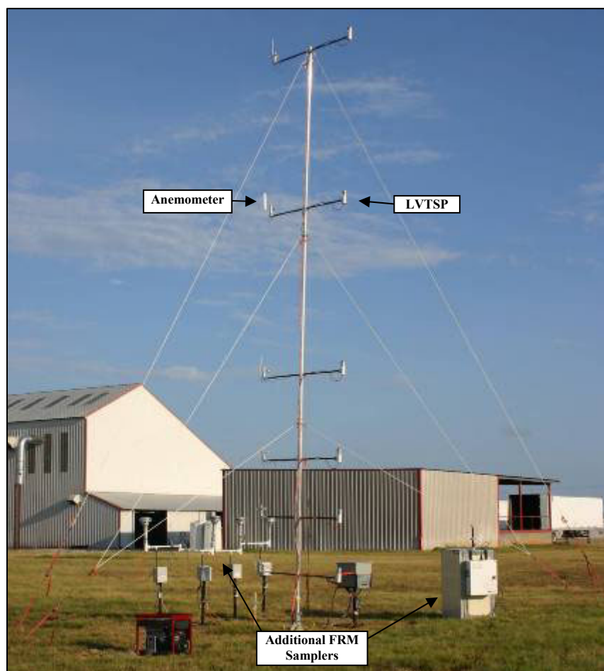
Figure 6. Configurations of ambient tower samplers with total suspended particulate sampler heads (LVTSP), wind anemometers, and additional stand-alone federal reference method samplers.
