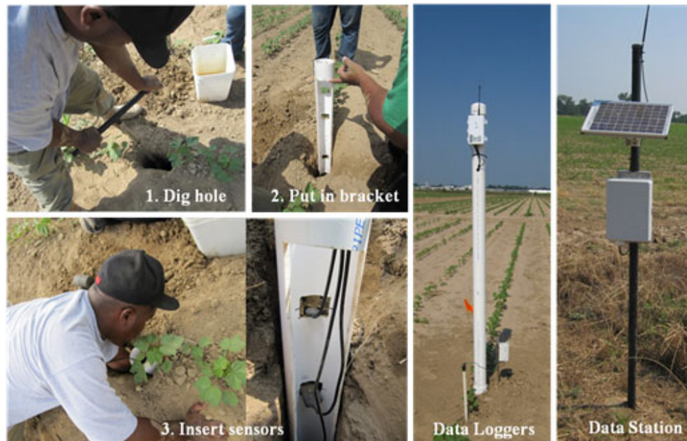
Figure 1. Show installation of soil moisture sensors, data loggers, and the data station.
