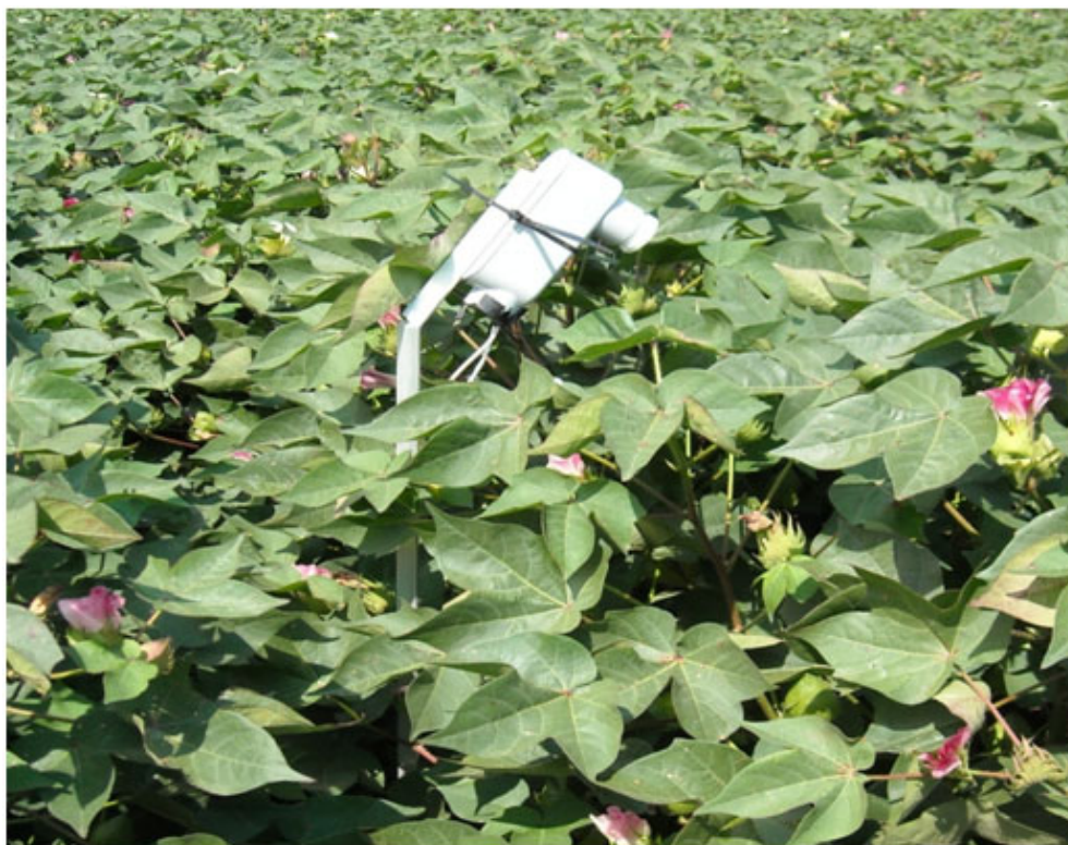
Figure 2. Infrared thermometer measuring cotton plant canopy temperature.
