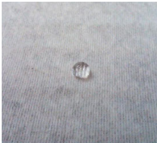
Figure 1 – A drop of water that almost indefinitely sits on the hydrophobic surface of the greige cotton nonwoven fabric bonded at 50/90/90 of water pressures.
