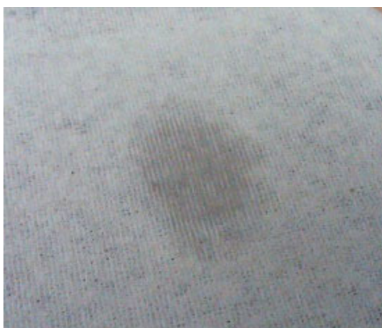
Figure 2 – A water drop that instantly diffuses (in less than 1 second) on the hydrophilic surface of the greige cotton nonwoven fabric bonded at 50/125/125 of water pressures.
