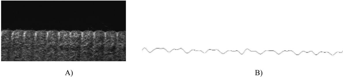
**Fig. 1** A) Roughness profile in the cross direction of tested fabric and B) corresponding slice after morphological operations and cleaning
