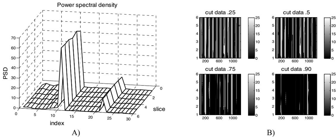
**Fig. 5** A) Periodogram for individual slices, B) surface extremes from indicator variable thresholds
