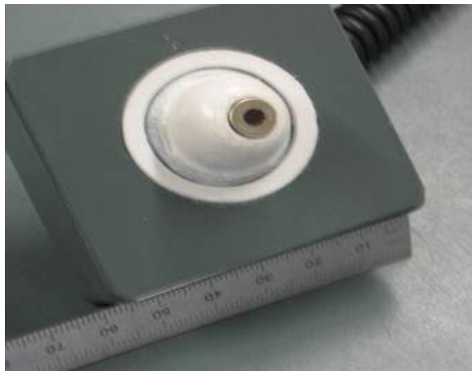
Figure 4. IR temperature sensor.
