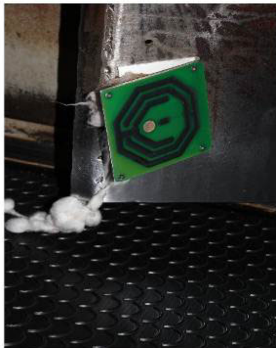
Figure 2. The Snail - Moisture sensor for lint and seedcotton
