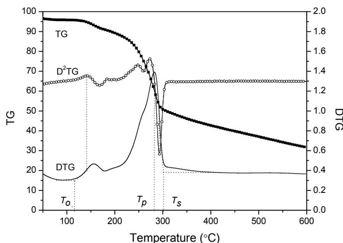
Figure 1. Thermal decomposition process of greige cotton nonwoven fabric treated with DAP and urea (D2U2) at a heating rate of 5 °C/min under nitrogen, and determination of thermal decomposition parameters.
