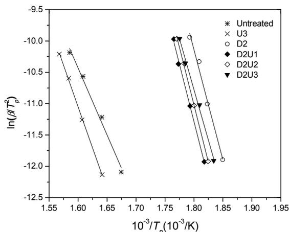
Figure 2. Plots of  $\ln(\beta/T_p^2)$  versus  $1/T_p$  for greige cotton nonwoven fabrics untreated and treated with DAP, urea, and mixtures of DAP and urea by Kissinger method.
