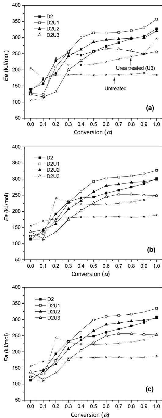
Figure 4. A variation of activation energy,  $E_a$ , as a function of conversion,  $\alpha$ , for untreated and treated greige cotton nonwoven fabrics: (a) Friedman method, (b) Flynn-Wall-Ozawa method, (c) modified Coats-Redfern method.
