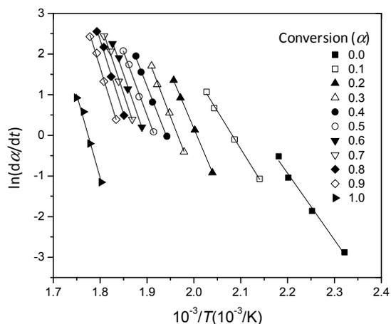
Figure 3. Iso-conversion plots of  $\ln(d\alpha/dt)$  versus  $1/T$  for greige cotton nonwoven fabric treated with DAP (D1) by Friedman method.
