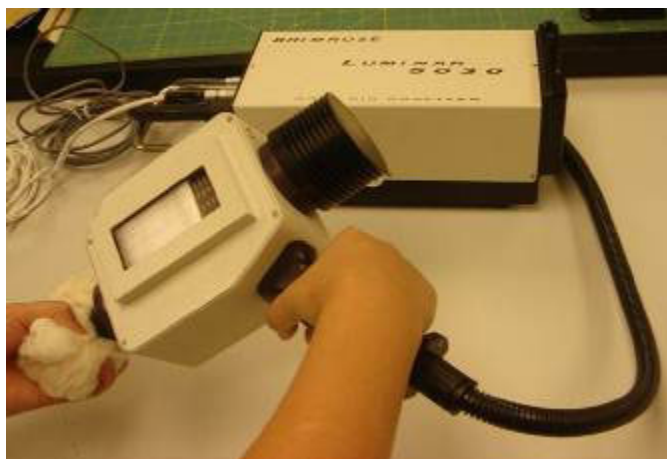
Figure 1. Brimrose Luminar 5030 portable NIR analyzer
