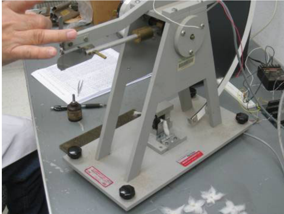
Figure 1. Fiber-seed attachment force tester just before releasing the pendulum. Pendulum arm locked in raised position and sample cartridge in place. Note the prepared seed with four bundles in the lower portion of the picture.
