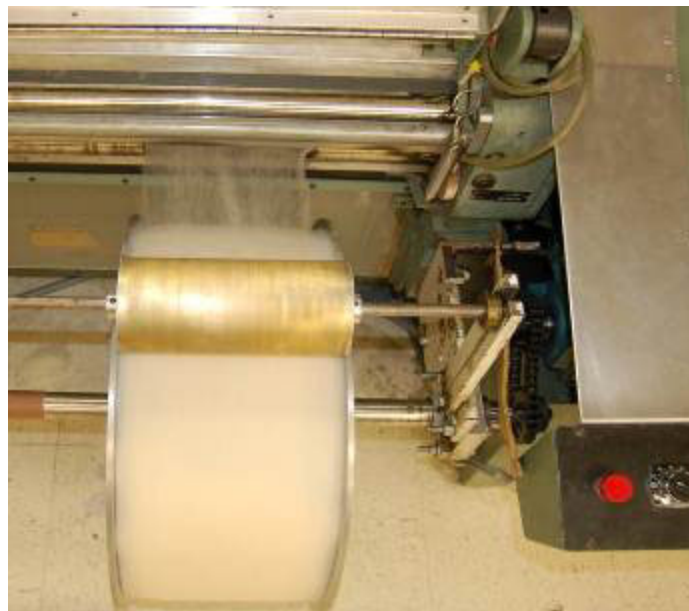
Figure 3. Card web collection system on mini-scale equipped card
