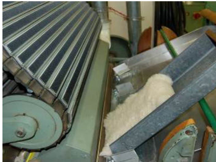
Figure 2. Tray feed system on mini-scale equipped card
