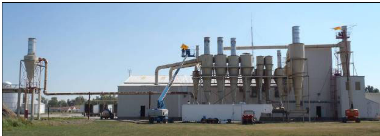
Figure 2. Stack sampling at the Missouri cotton gin.
