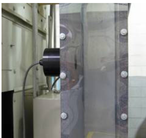
Figure 3. The mass-flow sensor installed on a duct behind gin stand to measure lint-flow at Cotton Ginning Research Unit in Stoneville, MS.
