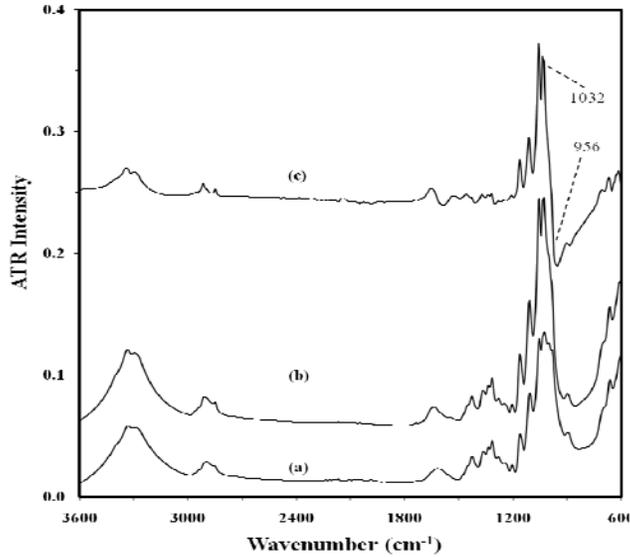
Figure 4. Typical FT-MIR spectra of mature (a) and immature (b) cotton fibers, and also difference spectrum (c, spectrum (b) – (a)). Spectra (b) and (c) were shifted vertically for direct comparison.
