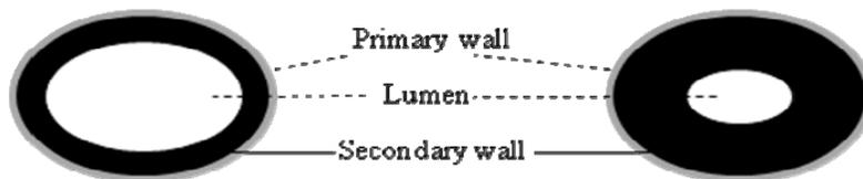
Figure 1. Schematic of immature (left) and mature (right) fiber cross-sections
