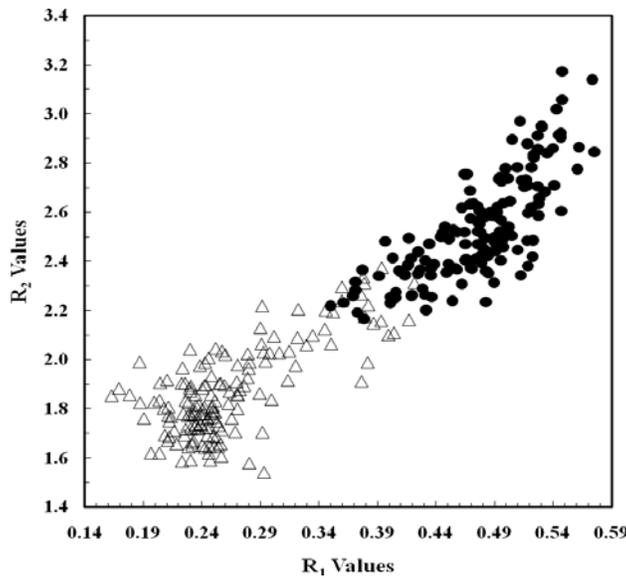
Figure 5. Plot of  $R_1$  vs.  $R_2$  values from seed cottons, immature ( $\Delta$ ) and mature ( $\bullet$ ).
