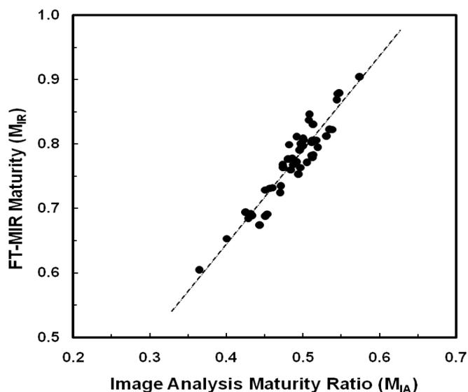
Figure 6. Relationship between  $M_{IA}$  from image analysis and  $M_{IR}$  from FT-MIR measurement.
