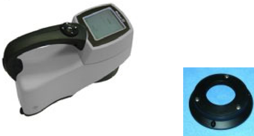
Figure 2. HunterLab MiniScan EZ (MSEZ) portable spectrophotometer and glass-covered 30 mm sampling port
