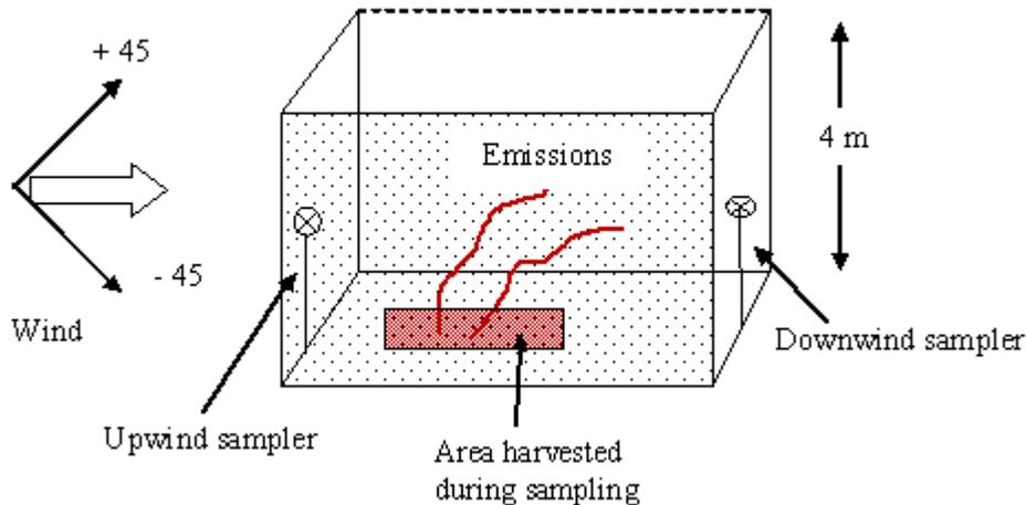
Figure 1. Schematic of the Flocchini box model
