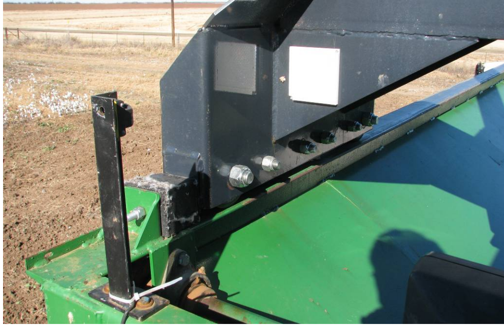
Figure 2. Photoelectric sensor and reflector for detecting cotton on sides of module builder.
