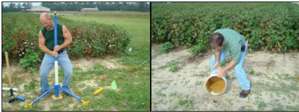
Figure 1: Probe installation techniques: Direct (left) and Slurry (right)
