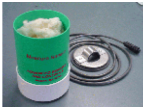
Figure 2. ASCI desk top moisture sensor containing a density sensor on board.
