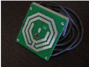
Figure 1. ASCI new moisture sensor containing a density sensor on board.
