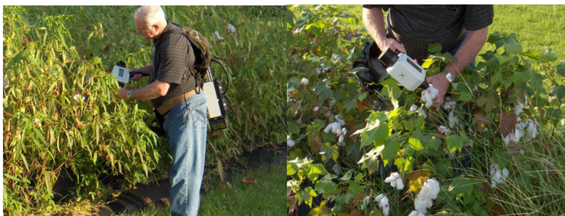
Figure 1. Field Analyses of Cotton Fiber Properties by Near Infrared (NIR) Spectroscopy. (Rodgers)
