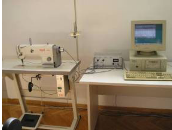
Figure 6. Instrument for measuring sewing needle penetration forces.
