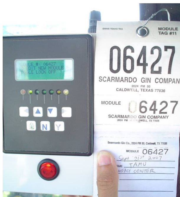
Figure 2. Module number being input into module builder subsystem before the module was built.
