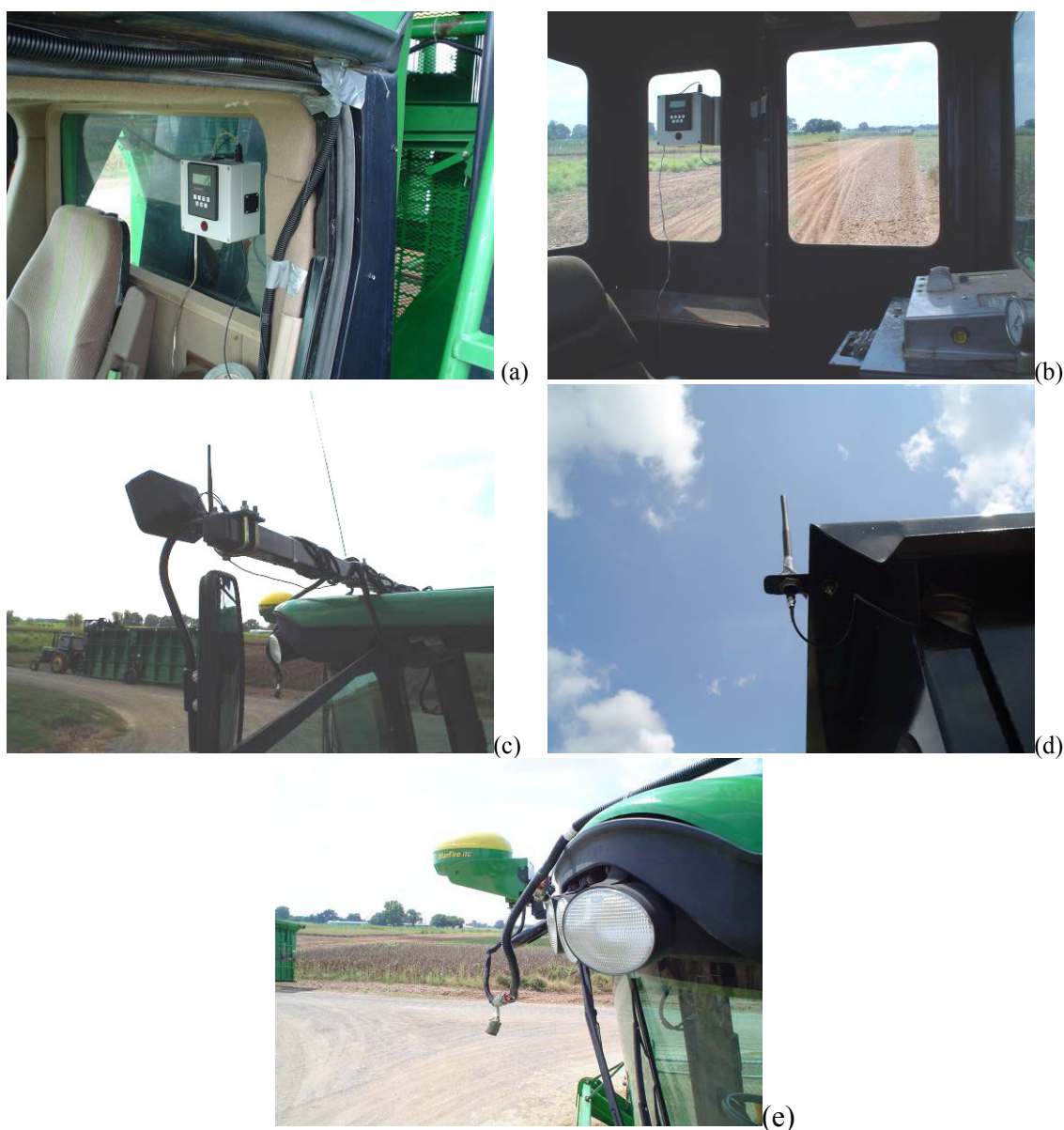
Figure 1. System installation in field test 2: (a) harvester subsystem in picker cab, (b) module builder subsystem in module builder cab, (c) wireless antenna on picker's light bar, (d) wireless antenna atop module builder cab, and (e) John Deere harness cable connecting Starfire1 to harvester subsystem.
