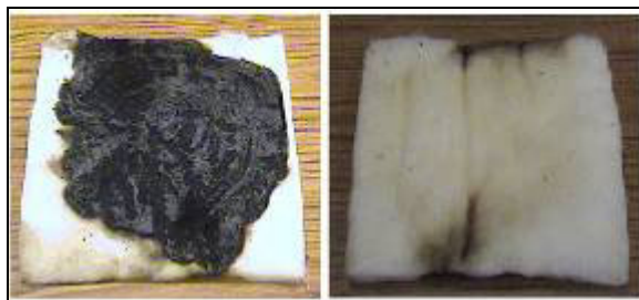
Figure 2 Sample Pad after the TB604 Test (Char on the fire side and change in color on other side)
