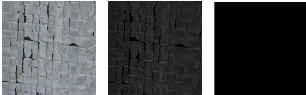
Figure 5. a) A small region of a module cover, b) the same region with back light applied, c) binary image after automatically pinhole detection.
