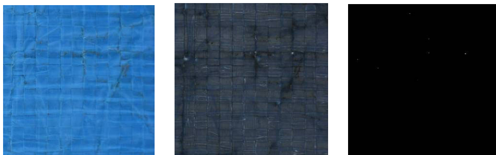
Figure 6. a) A small region of a module cover, b) the same region with back light applied, c) binary image after automatically pinhole detection (pinholes are present, although they may not be visible due to image resolution).
