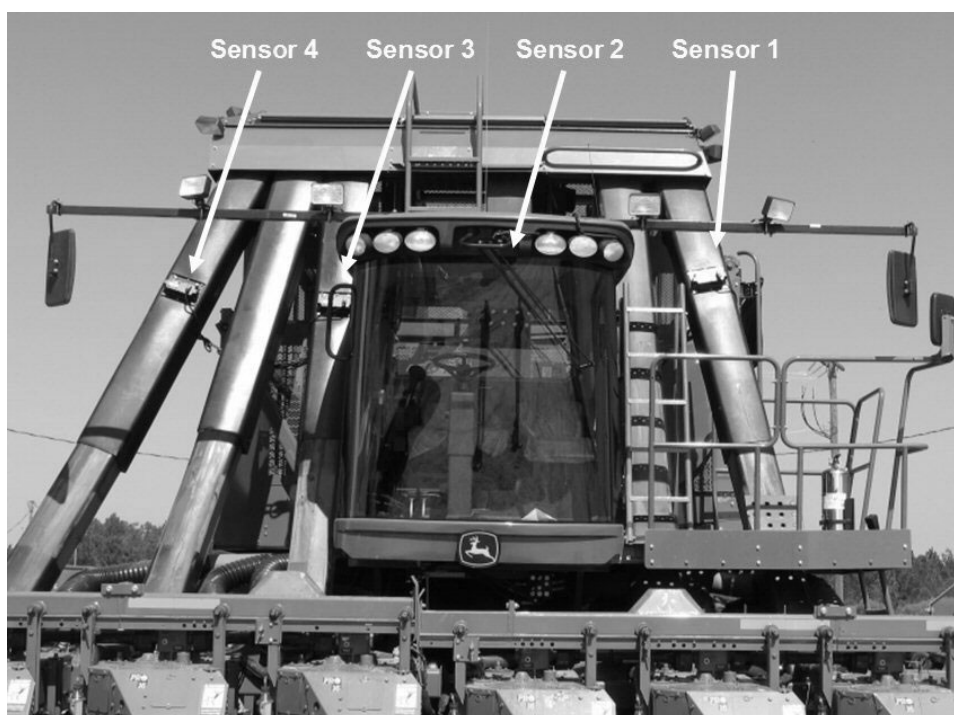
Figure 1. Ag Leader cotton flow sensors installed on 9996 cotton picker.
