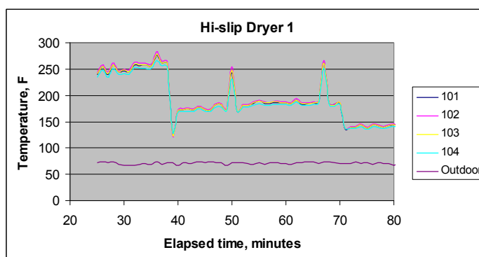
Figure 14. Temperature variation 10 feet (3 m) preceding the mixpoint of the hi-slip blow-box drying system 1. The numbers 101, 102, 103, and 104 refer to the code numbers for the thermocouples as recorded by the data acquisition system.
