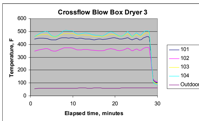
Figure 13. Temperature variation 10 feet (3 m) preceding the mixpoint of the crossflow blow-box drying system 3. The numbers 101, 102, 103, and 104 refer to the code numbers for the thermocouples as recorded by the data acquisition system.
