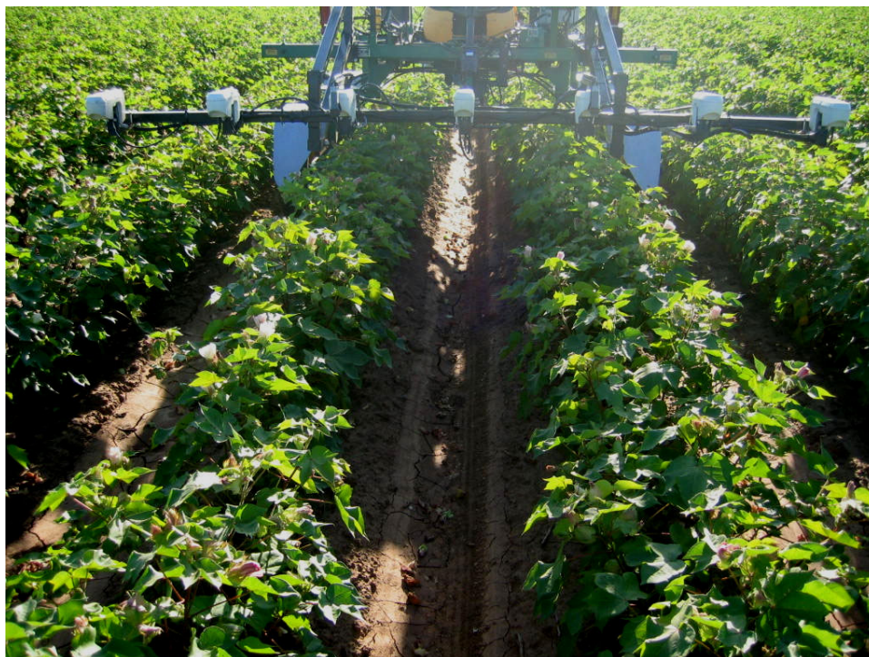
Figure 1. GreenSeeker® sensors and Ultrasonic sensors mounted on a boom
