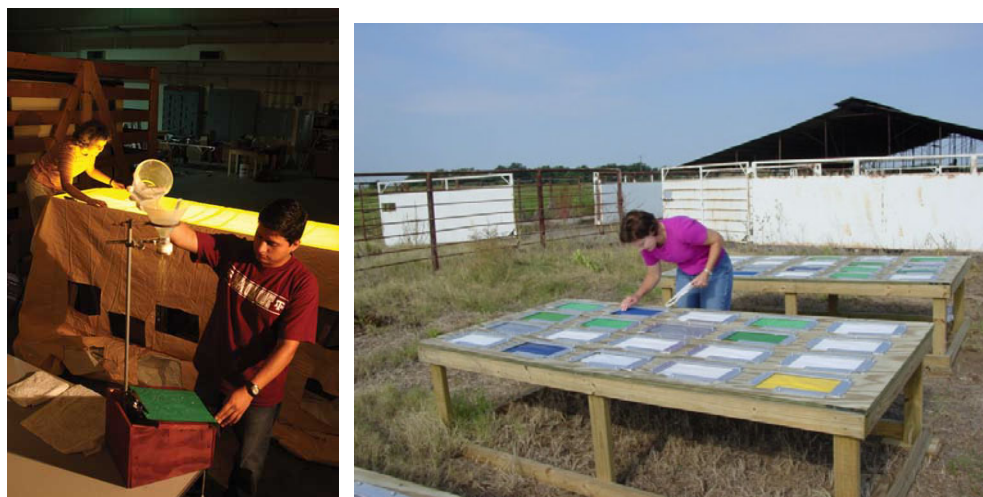
Figure 1a) Rainfall simulation in the foreground with light table evaluation in background; b) Tarp specimen in outdoor weathering racks.
