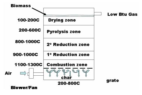
Figure 1. Schematic of an updraft gasifier (Capareda, 2006).
