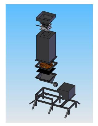
Figure 3. Downdraft gasifier (Capareda, 2006).
