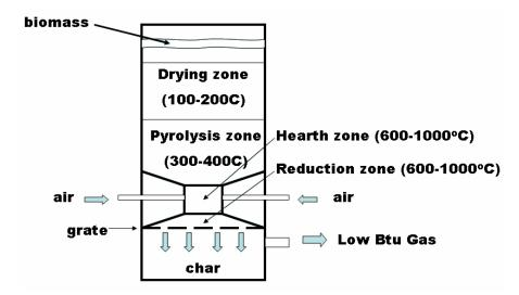
Figure 2. Schematic of a downdraft gasifier (Capareda, 2006).
