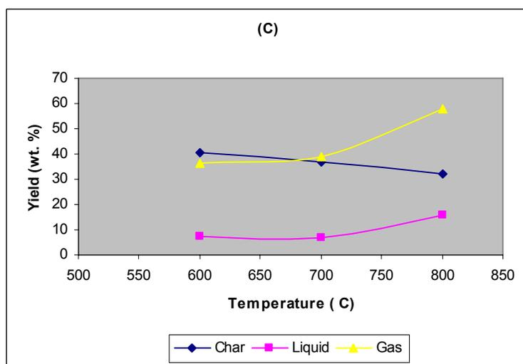
Figure 3. Product yields at different temperatures with pyrolysis time of 45 min.
