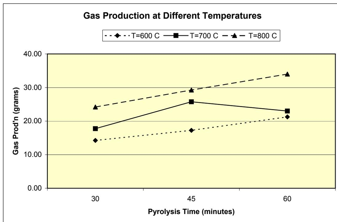
Figure 6. Gas production at different temperatures with increasing pyrolysis time.
