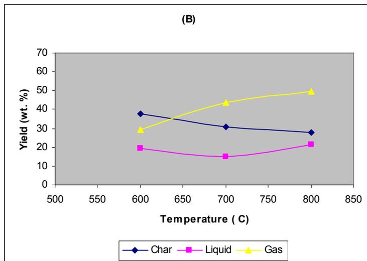
Figure 4. Product yields at different temperatures with pyrolysis time of 60 min.
