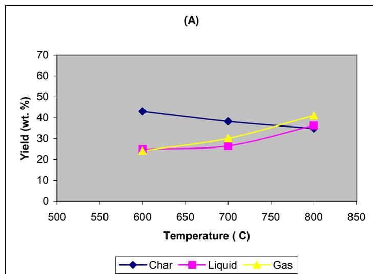
Figure 2. Product yields at different temperatures with pyrolysis time of 30 min.
