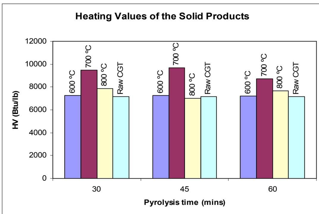
Figure 8. The measured heating values of the raw and pyrolyzed cotton gin trash samples.
