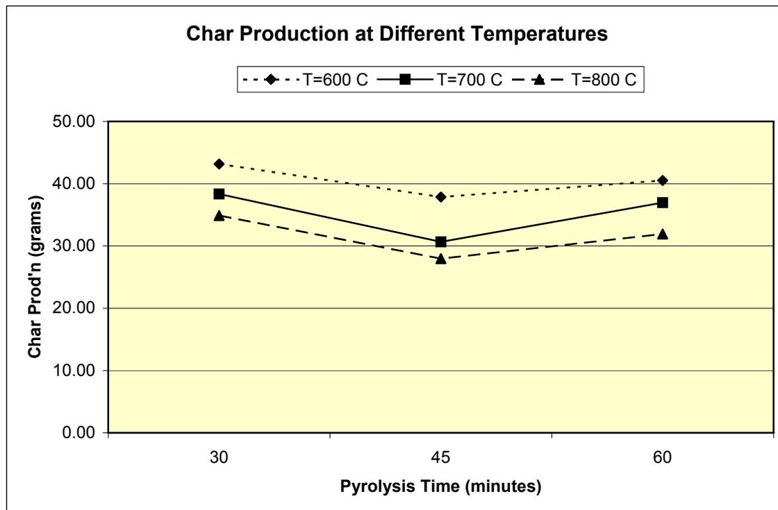
Figure 5. Solid (char) production at different temperatures with increasing pyrolysis time.
