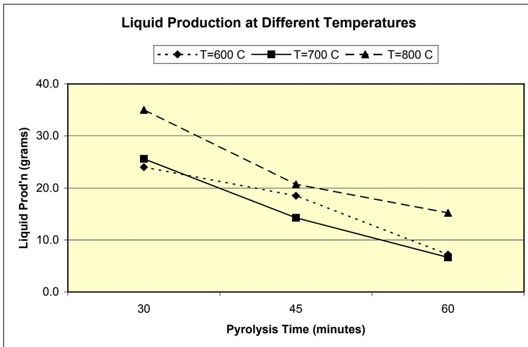
Figure 7. Liquid production at different temperatures with increasing pyrolysis time.
