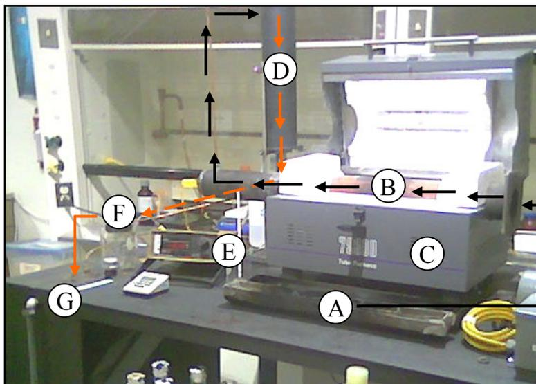
Figure 1. Pyrolysis setup used in the experiment showing the following parts: (A) steel container, (B) horizontal tube reactor, (C) horizontal tube furnace, (D) condenser, (E) thermocouple reader, (F) liquid collector/cold trap, and (G) displacement tanks.
