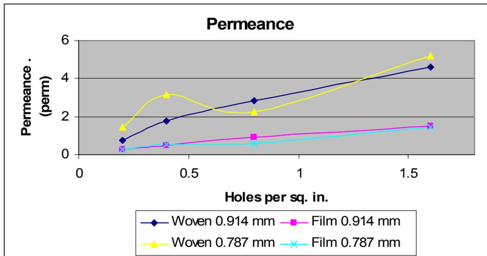
Figure 5. Permeance performance of WPP and PE versus hole density for both pin sizes.
