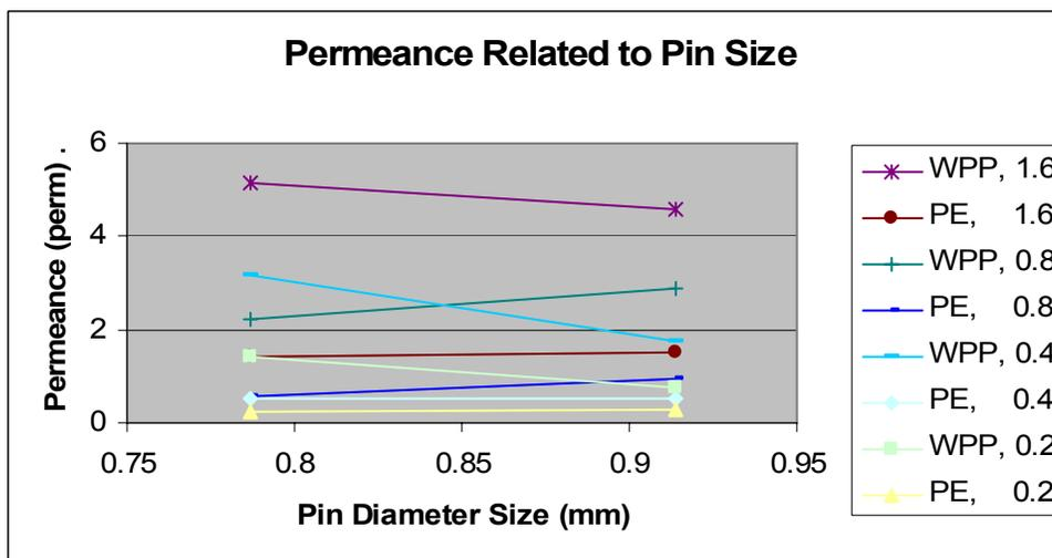
Figure 6. Permeance performance of WPP and PE versus pin size for four hole densities.
