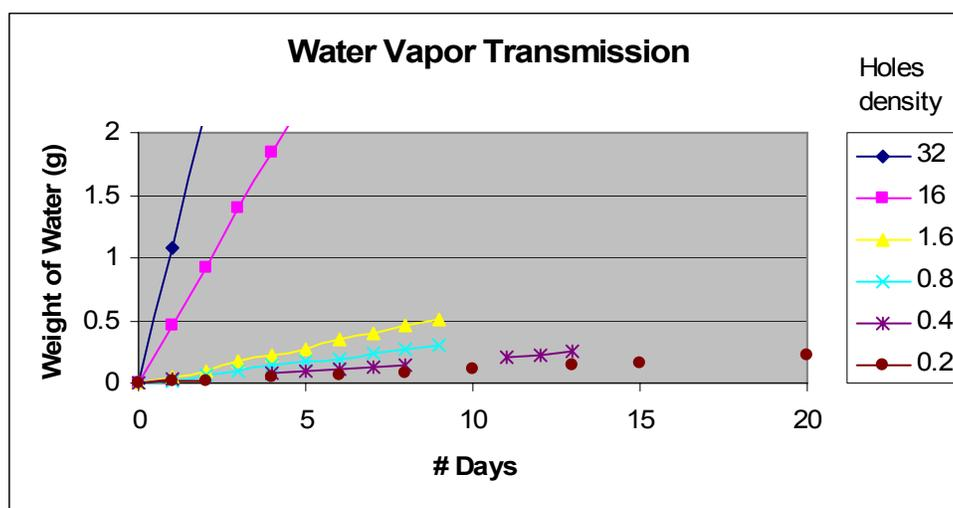
Figure 3. Water vapor transmission for polyethylene film bagging punched with pin size 0.914 mm.
