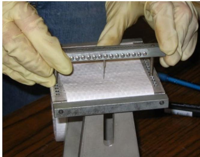
Figure 1. Pin punch and pin size 0.914 mm used to create uniform holes in WPP sample.
