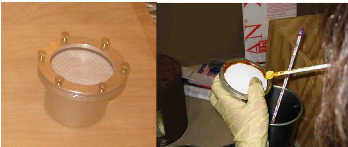
Figure 2. a) Vapometer with mechanical seal. b) Vapometer with WPP material being sealed with wax and rosin equal part mixture.
