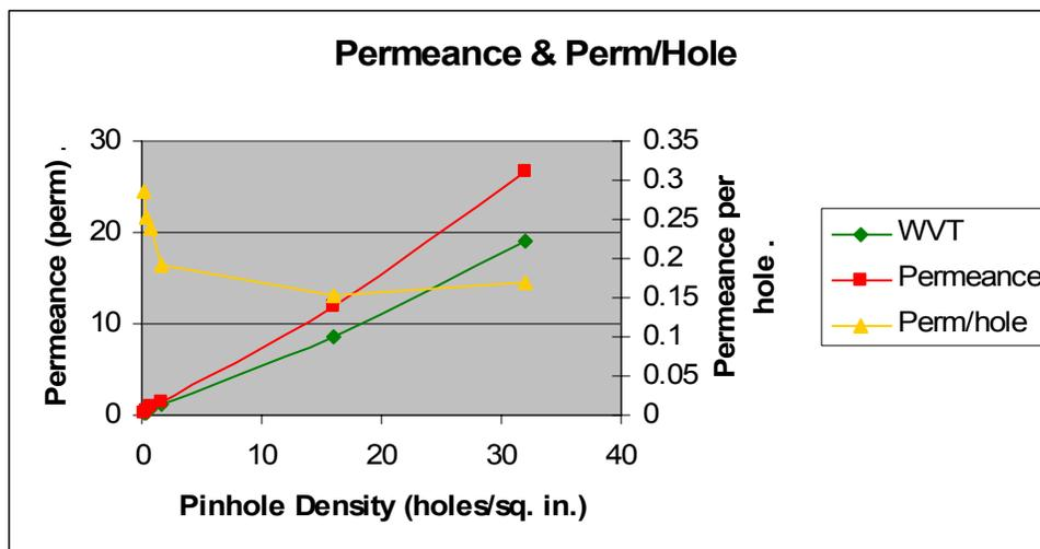
Figure 4. Permeance and permeance per hole for polyethylene film bagging punched with pin size 0.914 mm.
