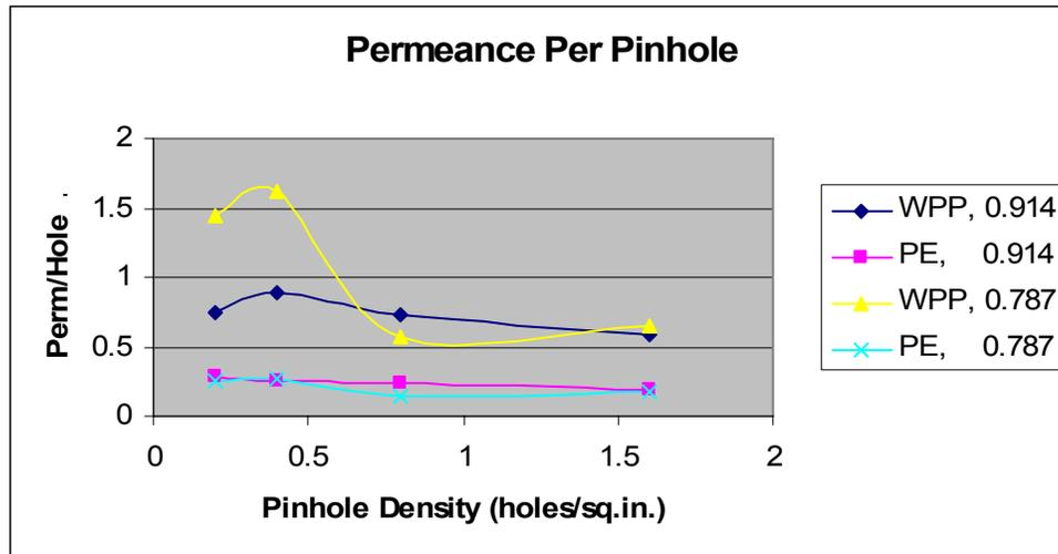
Figure 7. Permeance per pinhole performance of WPP and PE versus pinhole density for two pin sizes.
