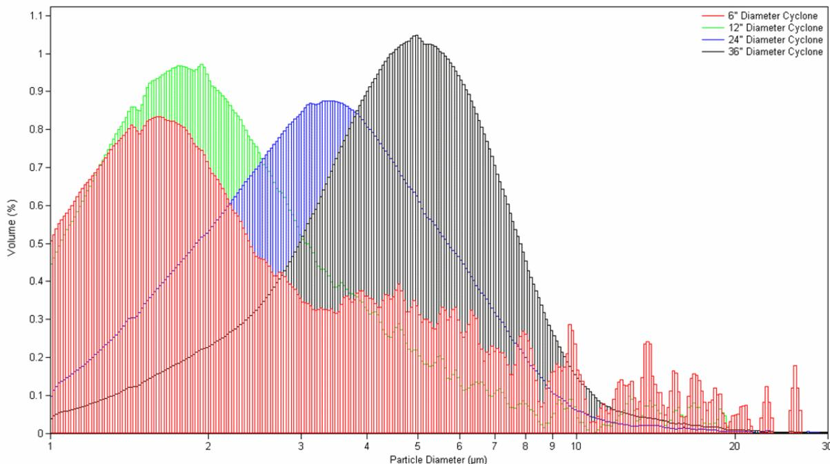
Figure 5. Average PSDs of PM collected on filters downstream of cyclones.
