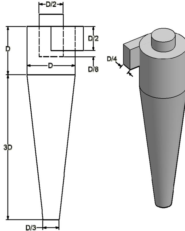
Figure 1. 1D3D cyclone configuration.
