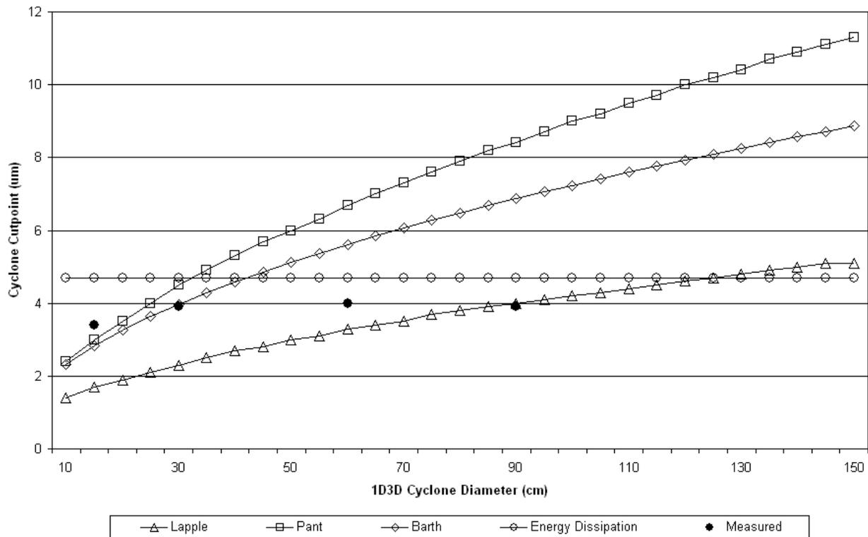
Figure 4. 1D3D cyclone cut point models and measured cut points.
