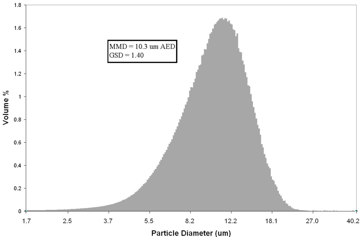
Figure 3. Particle size distribution of #5 microalumina used (in equivalent spherical diameter).
