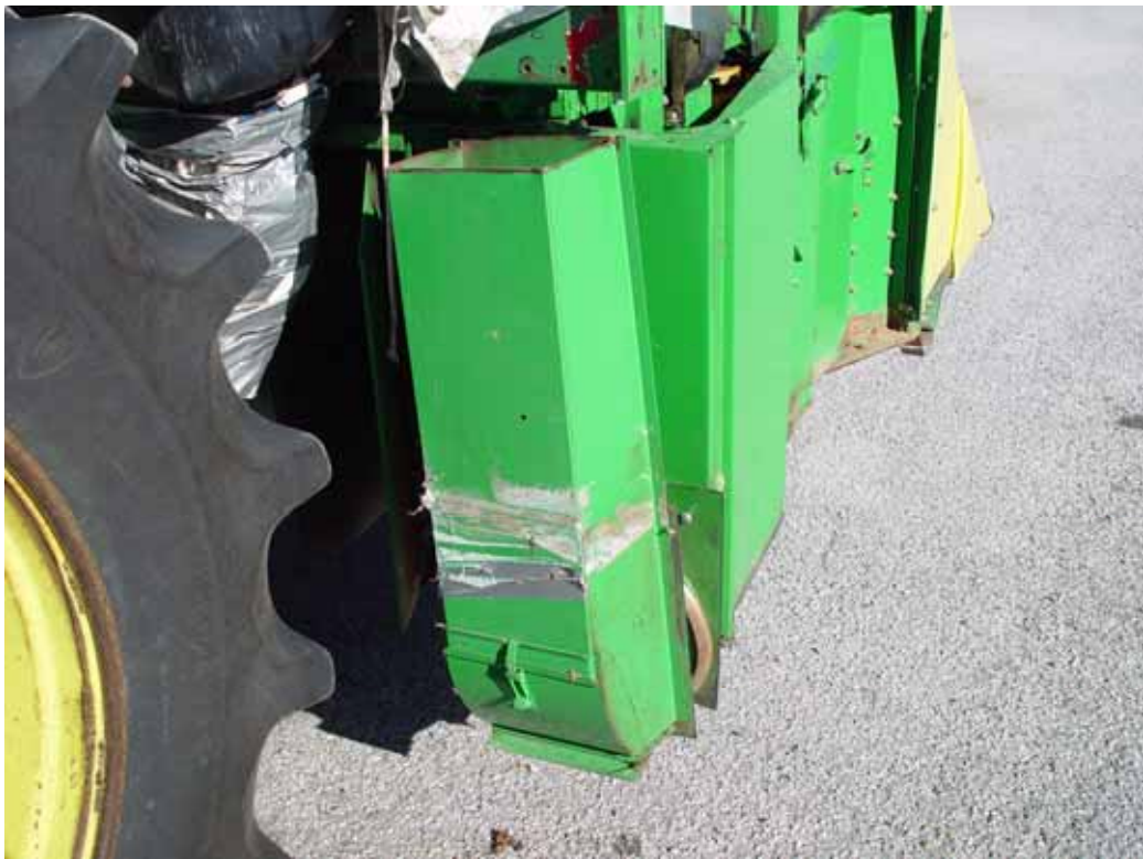
Figure 4: Swivel on back of picking unit for positioning row units.
