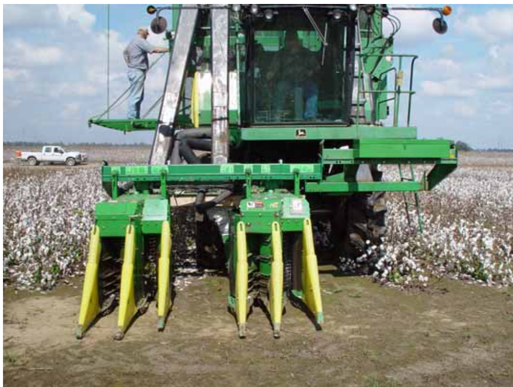
Figure 3: John Deere 9960 modified plot harvester set to harvest 15-inch 2X2 skip row.
