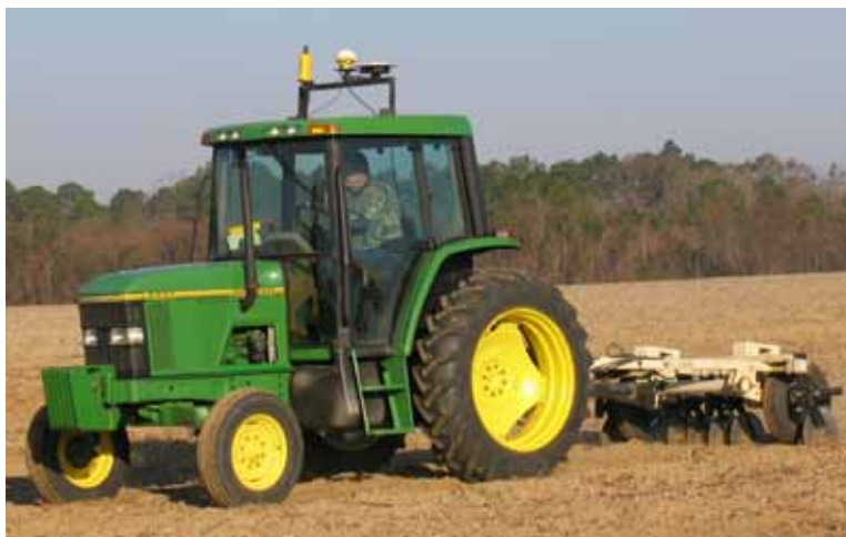
Figure 1. Veris 3100 soil EC sensor being pulled through soil. Tractor has RTK-GPS mounted for topographic mapping.
