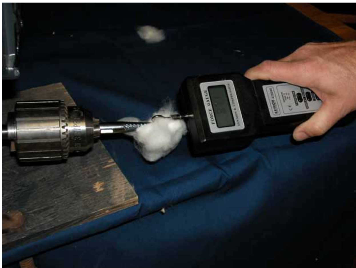
Figure 1. Pulling the cotton from the spindle using a force gage which records the peak force.
