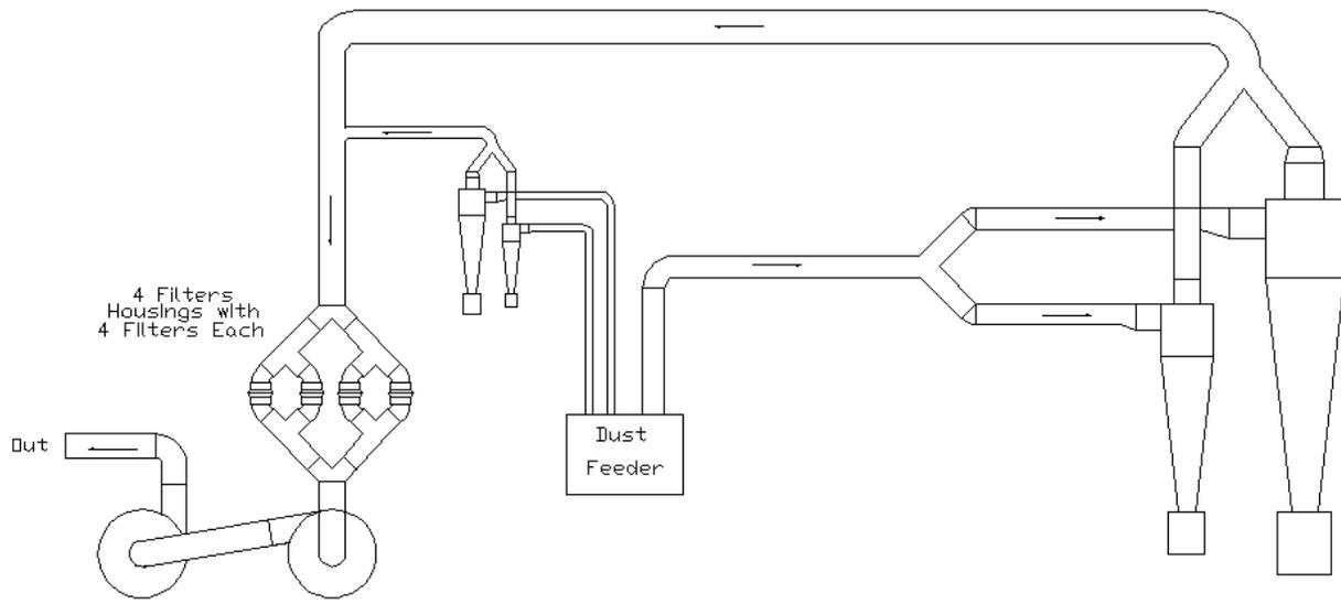
**Figure 3. Schematic of cyclone testing system.**
