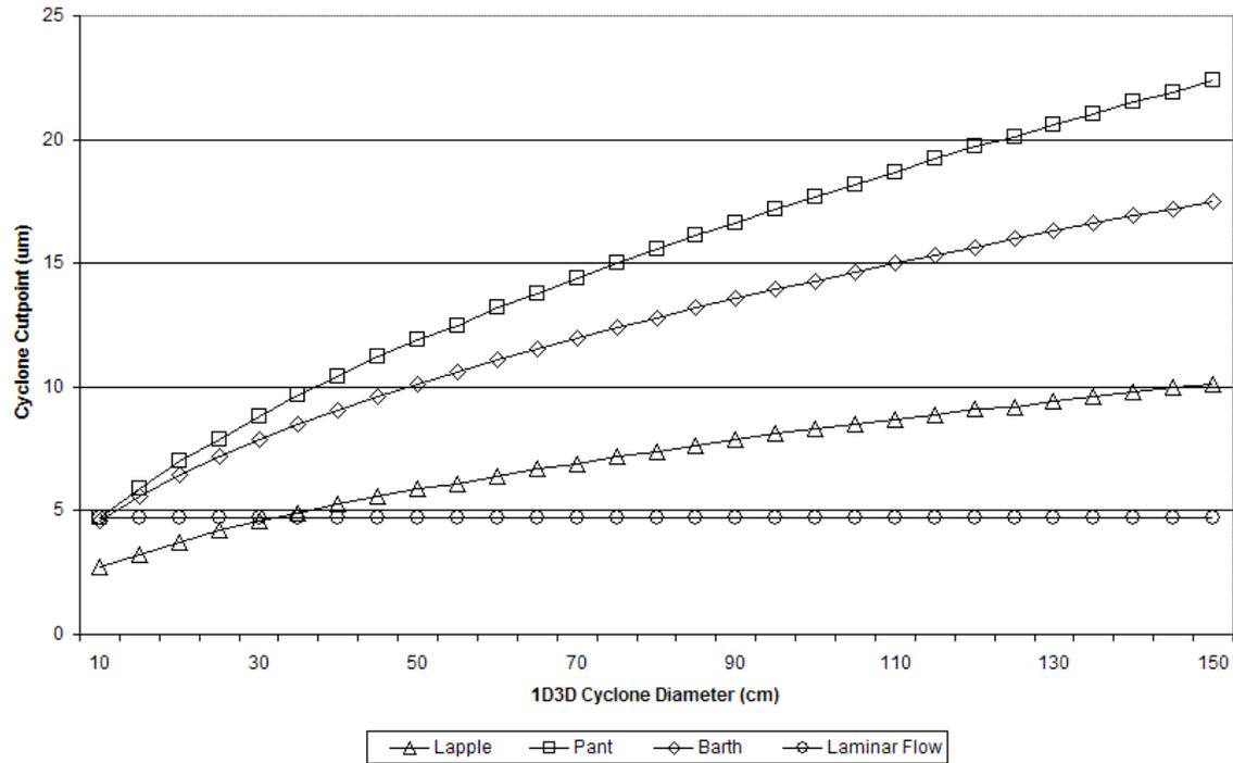
**Figure 2. 1D3D cyclone cut point models.**
