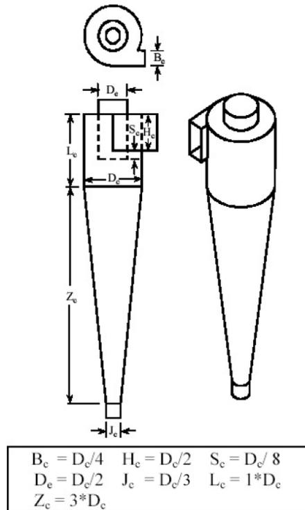
**Figure 1. 1D3D cyclone configuration.**
