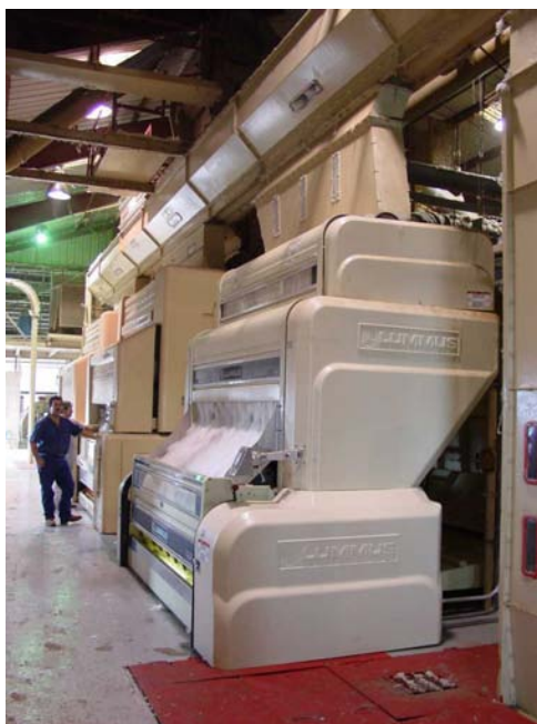
Figure 4. Installation of Lummus gin and feeder at Midway Gin Coop in Taft, Texas.
