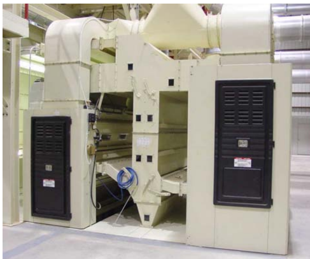
Figure 3. Tandem lint cleaning arrangement with Sentinel™ lint cleaner (left) and Model 108 lint cleaner (right).
