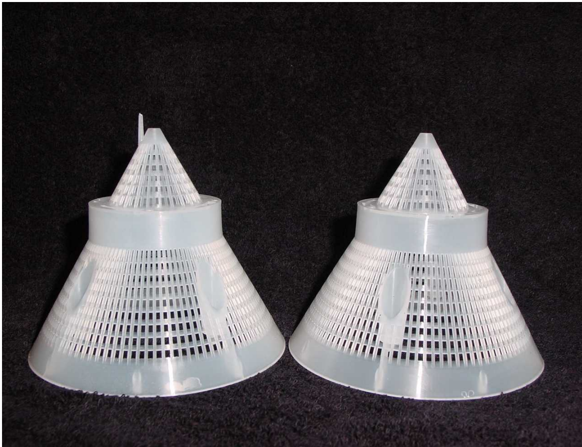
Figure 2. (L) Commercial cone. (R) Experimental cone with fill chimney removed.
