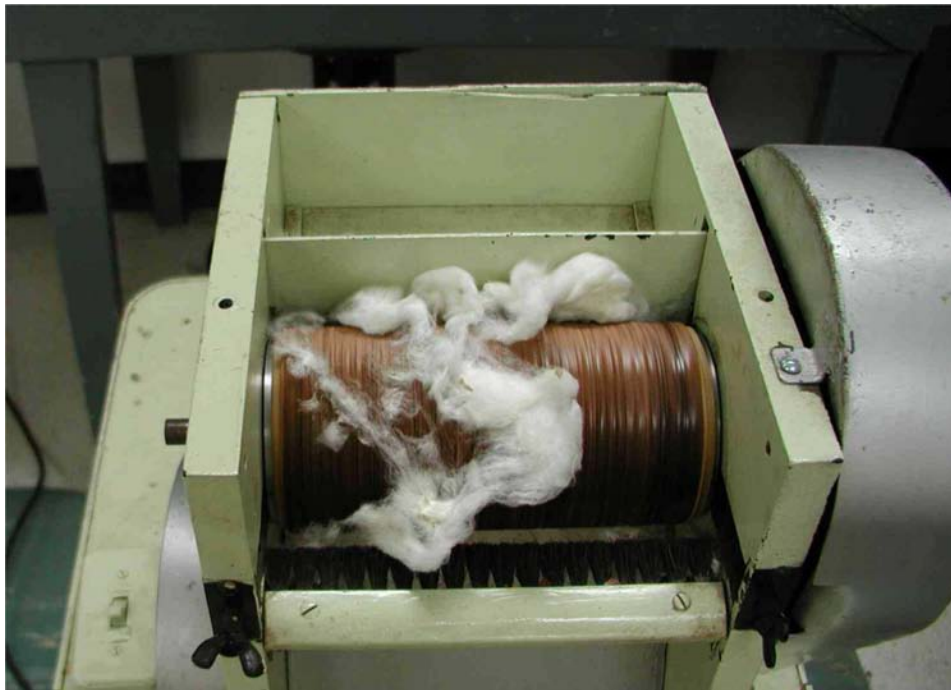
Figure 5. Laboratory roller gin in operation.
