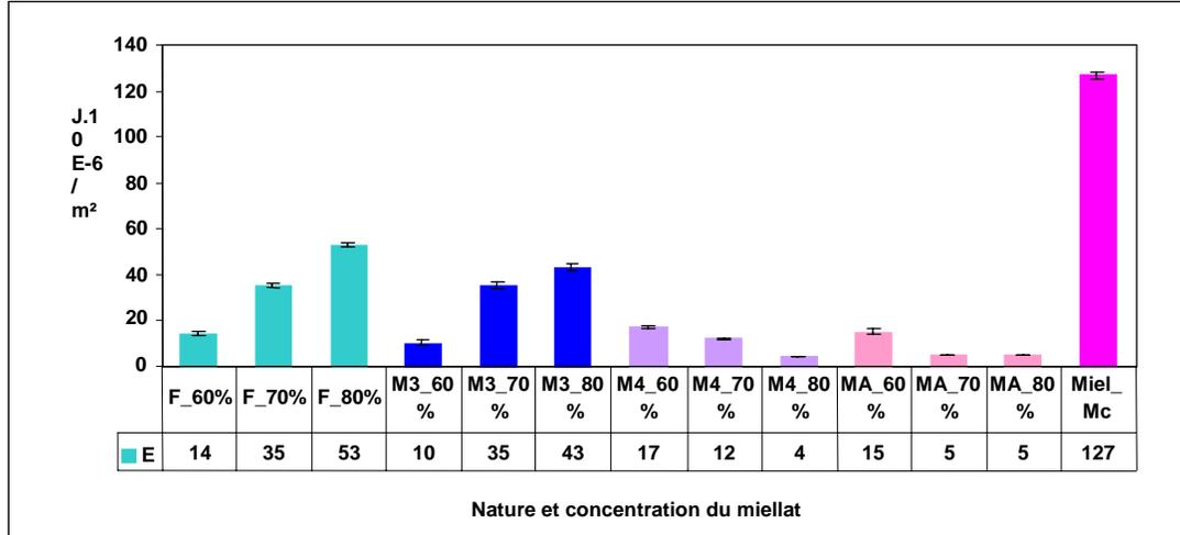
Figure 7. Adhesion energy vs. Type of sugar as a function of water content for Mosaic D. Adhesion energy J 10-6/m2
