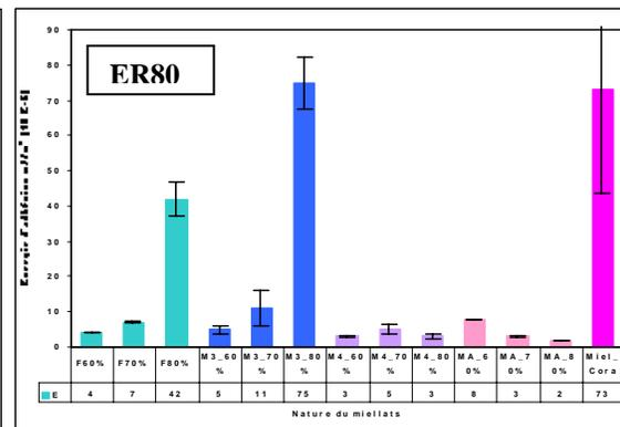
Figure 6. Adhesion energy vs. Type of sugar as a function of water content for HB55 and ER80
